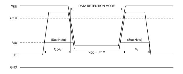
Note: When  $\overline{\text{CE}}$  is operating at the V<sub>IH</sub> level (2.4V), the standby current is given by I<sub>DDS1</sub> during the transition of V<sub>DD</sub> from 4.5 to 2.6V.
